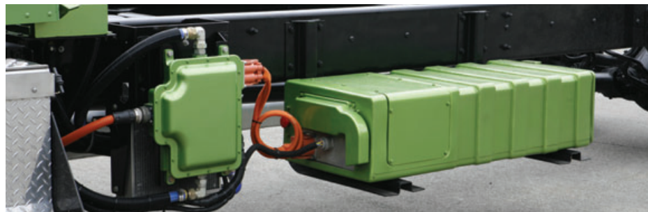
TOP: Primary components of the Hybrid system are a Hybrid Drive Unit (HDU), which combines a clutch, a nearly 60 horsepower motor/generator and automated manual transmission; the motor inverter/controller; the DC/DC converter (utility only); and a 340 volt lithium-ion battery pack.
